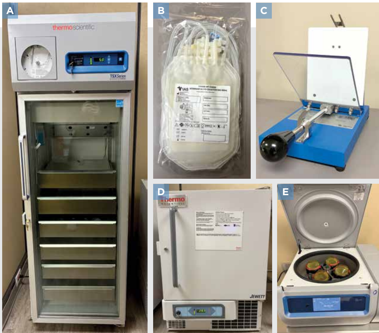
FIGURE 2. Essential supplies for blood component processing: (A) medical-grade blood refrigerator, (B) canine component processing bags, (C) plasma press, (D) plasma freezer, and (E) table top centrifuge.
