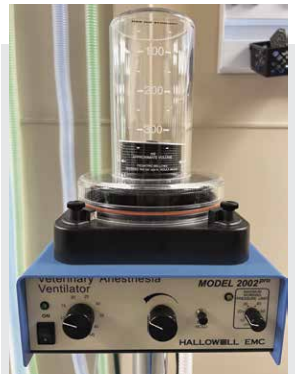
FIGURE 4. Surgical ventilator used for positive-pressure ventilation during anesthesia.
