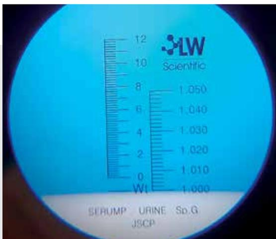
**FIGURE 7.** Calibrated refractometer scale of the Jorvet analog refractometer ([jorvet.com](http://jorvet.com)).
