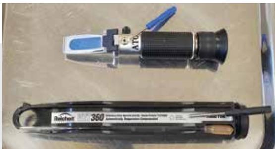
**FIGURE 8.** Calibration screw. While distilled water under the prism is viewed, the calibration screw is turned to adjust the calibration according to the refractometer instructions.
