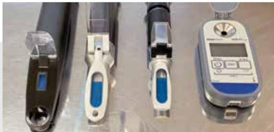
**FIGURE 2.** Various types of refractometers. Left to right: Reichert multispecies analog ([reichert.com](http://reichert.com)), Westover analog, Jorvet analog ([jorvet.com](http://jorvet.com)), Fisher digital ([fishersci.com](http://fishersci.com)).
