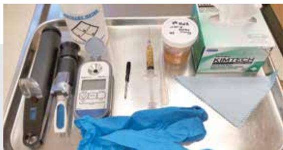
**FIGURE 6.** Materials required for measuring urine specific gravity: refractometer, distilled water, calibration screwdriver for analog models, urine sample, transfer pipette, laboratory optical tissue or a soft cloth, gloves, and natural or artificial light.
