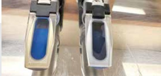
**FIGURE 9.** An adequate volume of urine is required. Right: Proper sample volume. Left: Inadequate sample volume. An inadequate sample volume will result in a blurred interface between the white and blue areas, leading to the potential for reporting inaccuracies. Either more sample can be applied to the prism or the cover can be gently pressed to ensure complete coverage of the prism with the sample.
