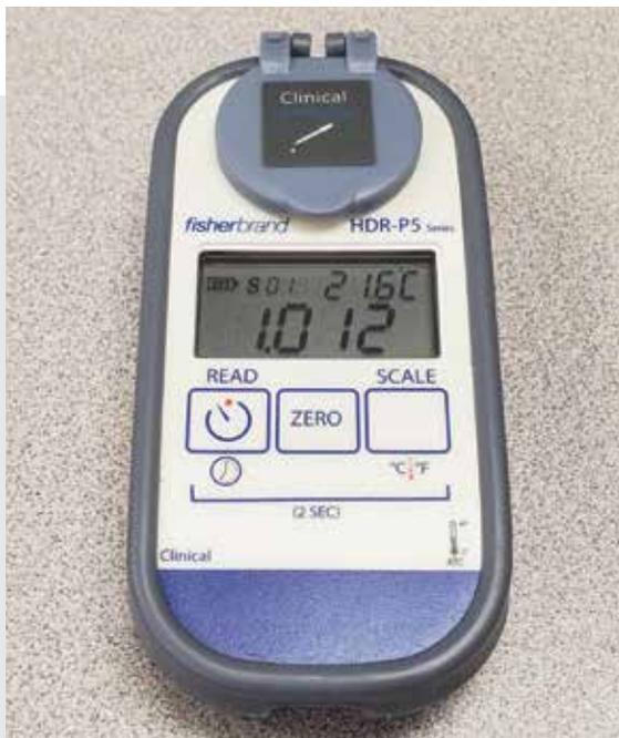
**FIGURE 10.** Isosthenuric specific gravity reading of 1.012 on a digital refractometer scale.
