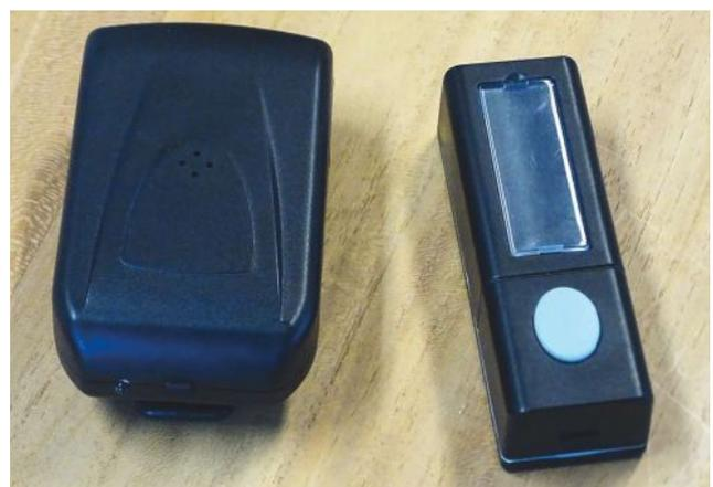
FIGURE 4. Wireless doorbell for client signaling.
